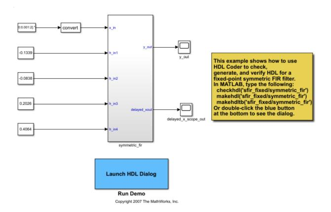
The top-level model generates 16-bit fixed-point input signals for the symmetric\_fir subsystem. The signal From Workspace block generates a test input or stimulus signal for the filter. The four Constant blocks provide filter coefficients. The Scope blocks are used in simulation, and do not generate HDL code.
