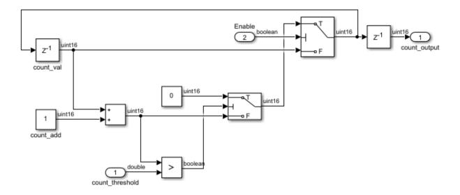
The model has two input ports, count\_threshold and Enable, and one output port, count\_output. When the Enable signal is logic high, the counter counts up from zero to the count\_threshold value and then wraps back to zero. When the Enable signal becomes logic low, the counter holds the previous value.
