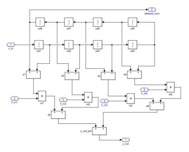
The fixed-point data types propagate through the subsystem. Inputs inherit the data types of the signals presented to them. Where required, internal rules of the blocks determine the output data type, given the input data types and the operation performed. The filter outputs a fixed-point result at the y\_out port, and also replicates its input after passing it through several delay stages at the delayed\_x\_out port.
